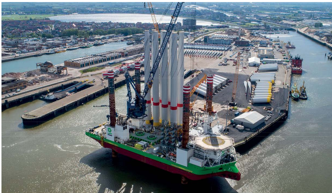
Transport of WTG Components via Jack-Up Vessel
