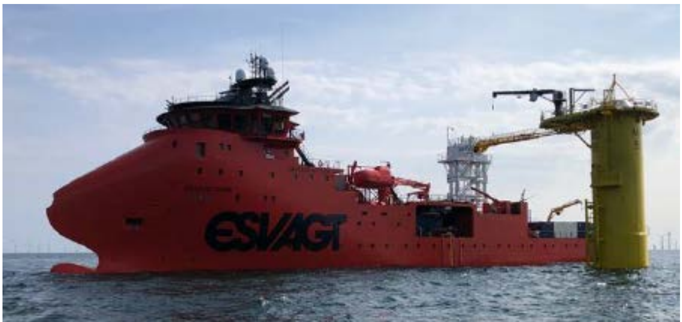
Example Service Operation Vessel (SOV)
